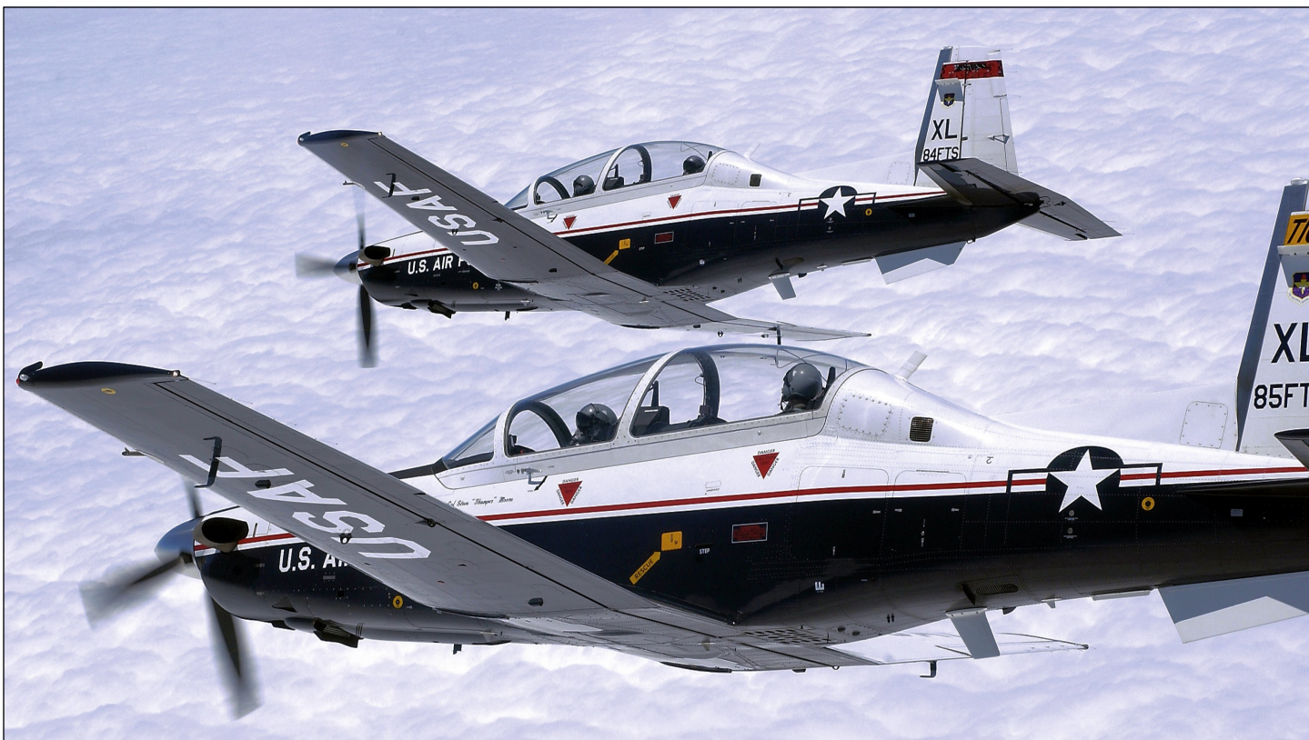
The T-6A Texan II is a single-engine, two-seat primary trainer designed to train Joint Primary Pilot Training, or JPPT, students in basic flying skills common to U.S. Air Force and Navy pilots. Produced by Raytheon Aircraft, the T-6A Texan II is a military trainer version of Raytheon's Beechcraft/Pilatus PC-9 Mk II. (U.S. Air Force photo)
